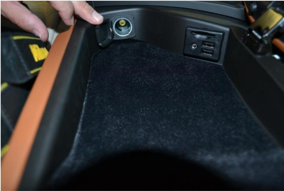
There is 1 Aux. power port located in the rear of the vehicle on the driver's side above the storage compartment for powering a battery maintainer.
