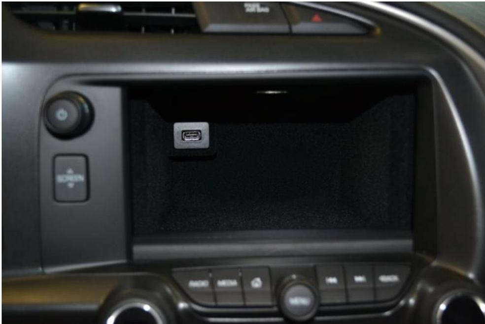
1 Aux. power port, 1 3.5 mm input jack, 2 USB ports and 1 SD Media slot in the center console
